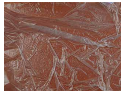
Marble effect: foil on the surfacer surface
